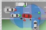
360° monitoring system with integrated lane and object detection
