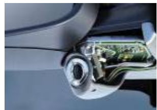
First camera-based blind spot detection system
