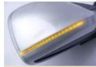
First light guide style turn signal (Audi Q7)
