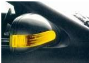
First turn signal in exterior mirror (Mercedes-Benz)
