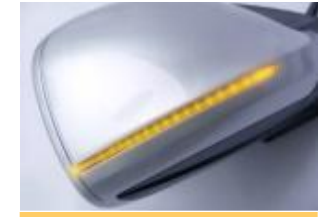
First light guide style turn signal (Audi Q7)
