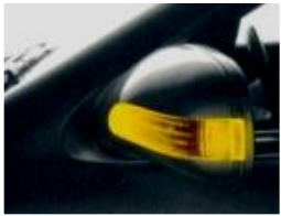
First turn signal in exterior mirror
