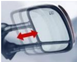
First combined power telescopic and power folding mirror
